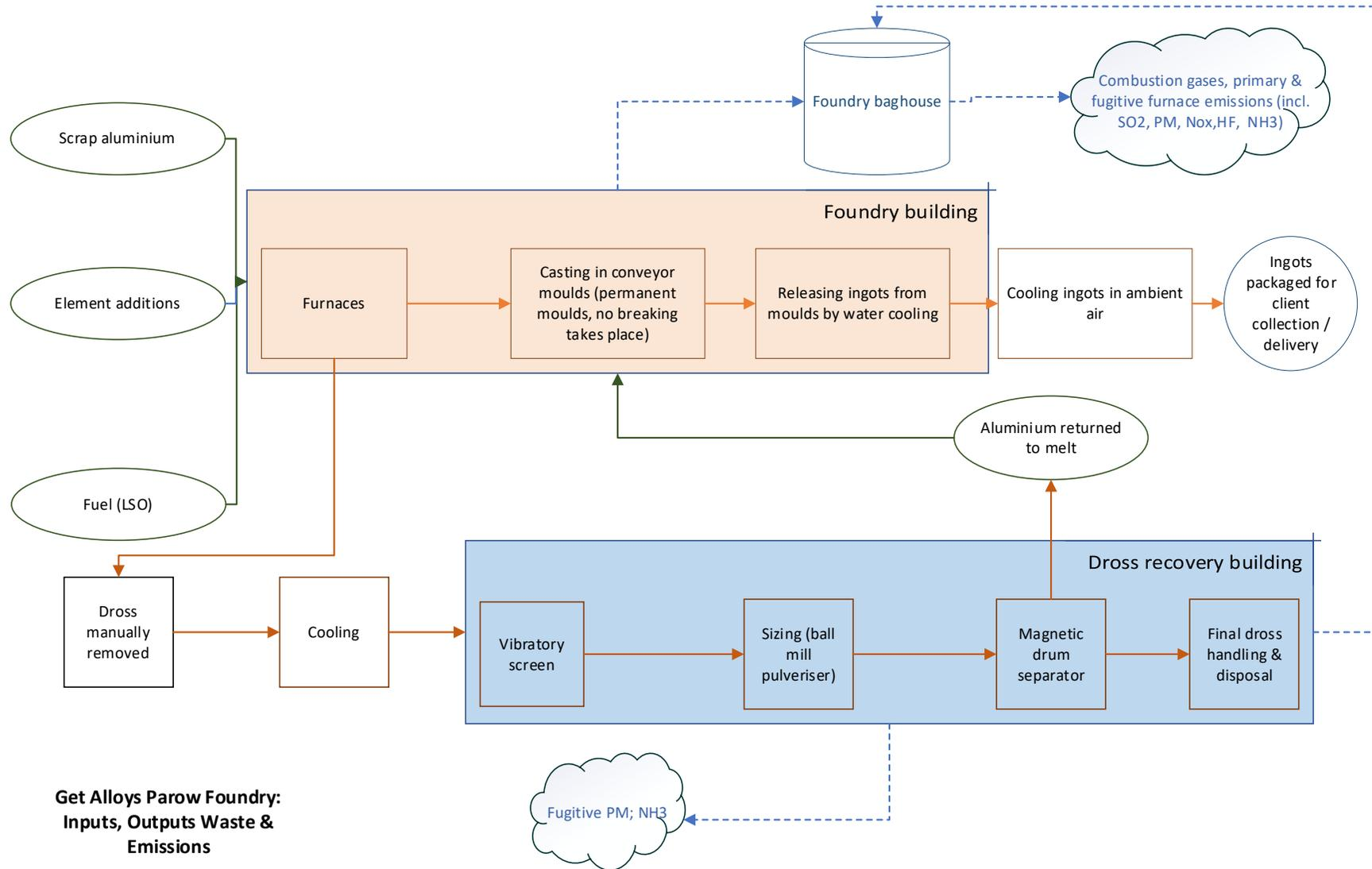
Figure 3 Dross management procedure process flow diagram
